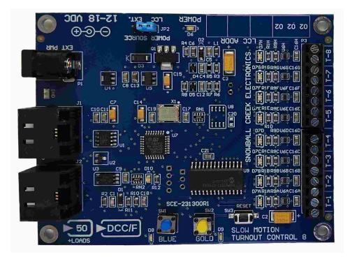
Slow-motion turnout control for an LCC or DCC network
